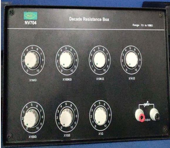
A photograph of a black electronic device labeled "Decade Resistance Box NV704". It features eight rotary knobs arranged in two rows of four. Each knob is labeled with ranges: X1MΩ, X100KΩ, X10KΩ, X1KΩ, X100Ω, X10Ω, X1Ω, and X1MΩ. A small digital display is visible above the knobs. An output terminal block with red and green wires is located on the right side.                                                                 |
