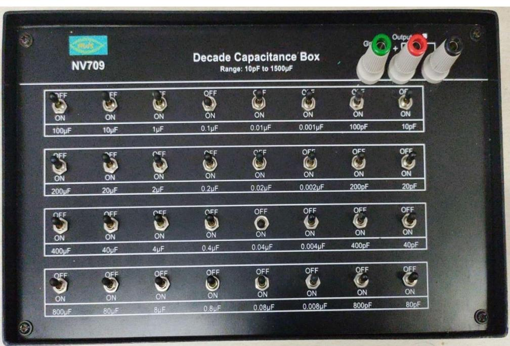
A photograph of a black electronic device labeled "Decade Capacitance Box NV709". It has four rows of four rotary switches each, labeled from top to bottom: 100µF, 10µF, 1µF, 0.1µF; 0.01µF, 0.001µF, 100pF, 10pF; 200µF, 20µF, 2µF, 0.2µF; 0.02µF, 0.002µF, 200pF, 20pF; 400µF, 40µF, 4µF, 0.4µF; 0.04µF, 0.004µF, 400pF, 40pF; and 800µF, 80µF, 8µF, 0.8µF. On the right side, there are three output terminals labeled GND, +, and -. |
