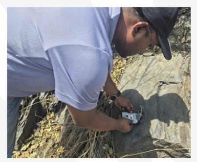
Fig 2: Use of Brunton compass for measuring Dip
